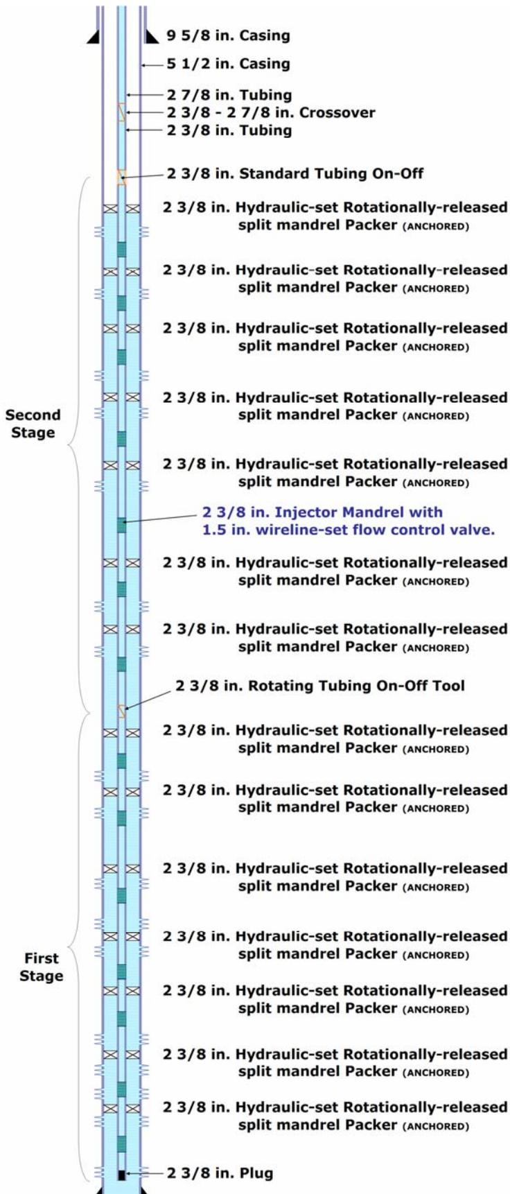
Fig. 10 – Hydraulic-set rotationally-released completion with split mandrel packers
