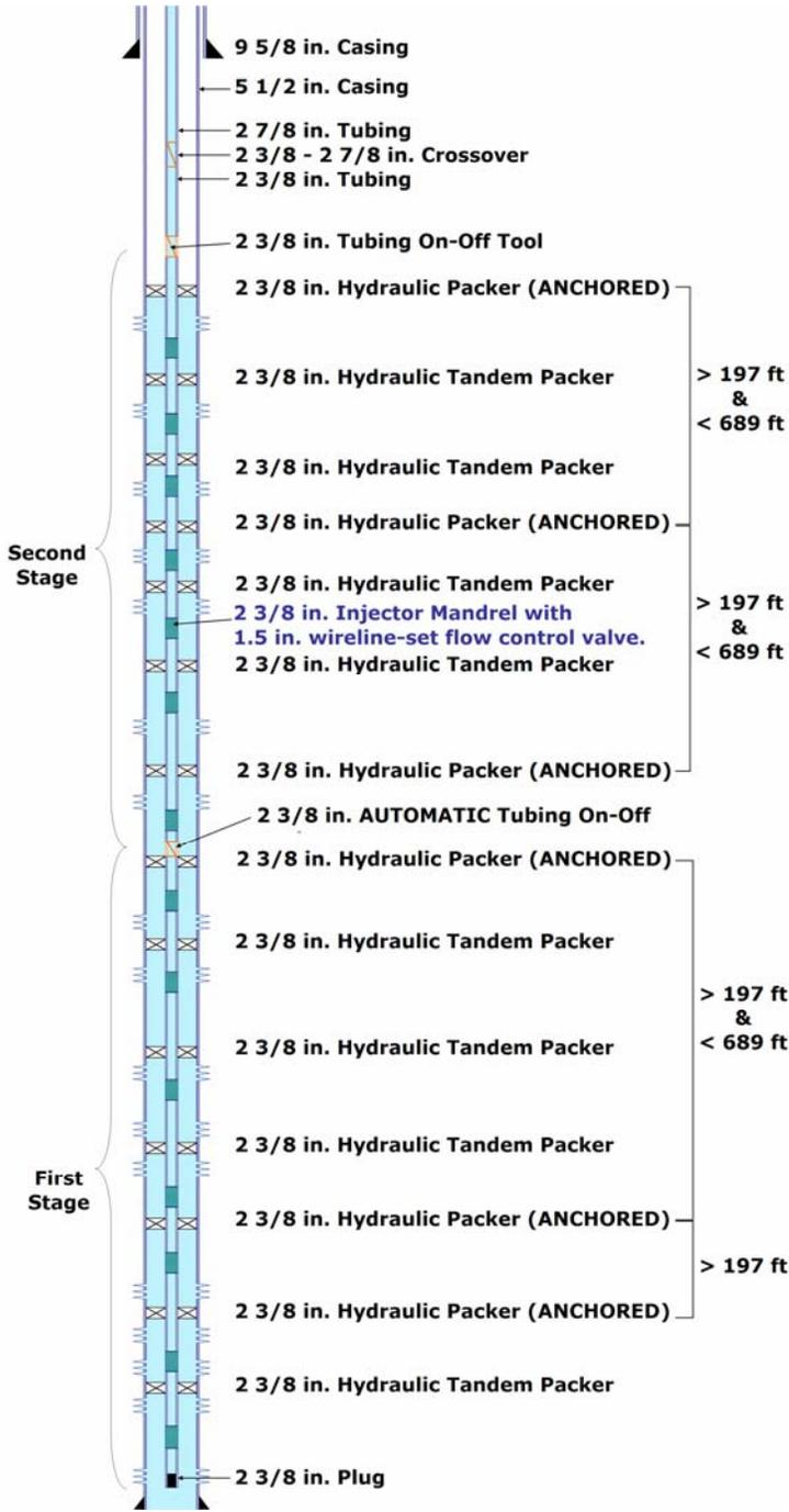
Fig. 8 – Hydraulic Packers Completion; multiple anchored points; two stages; 1 tubing run
