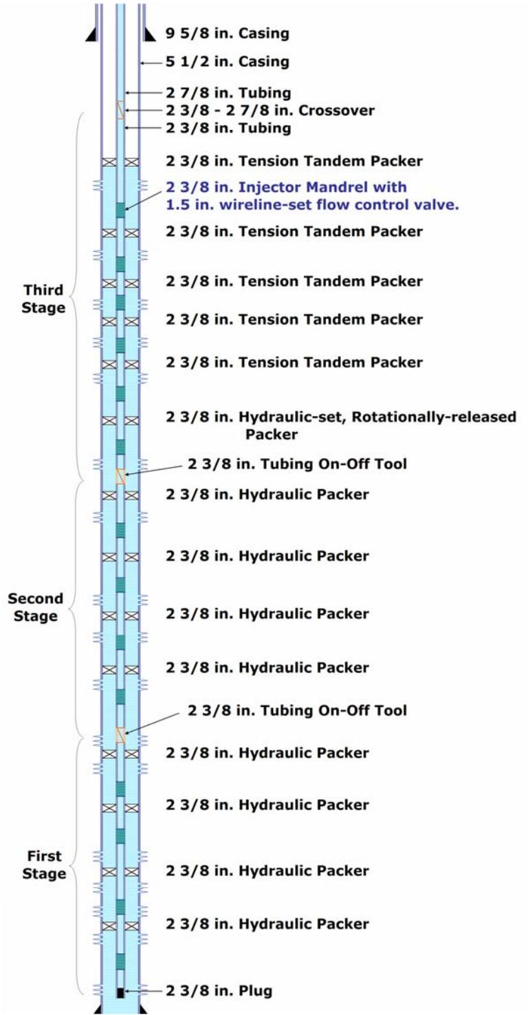
Fig. 5 – Mechanical and Hydraulic Packers Completion
