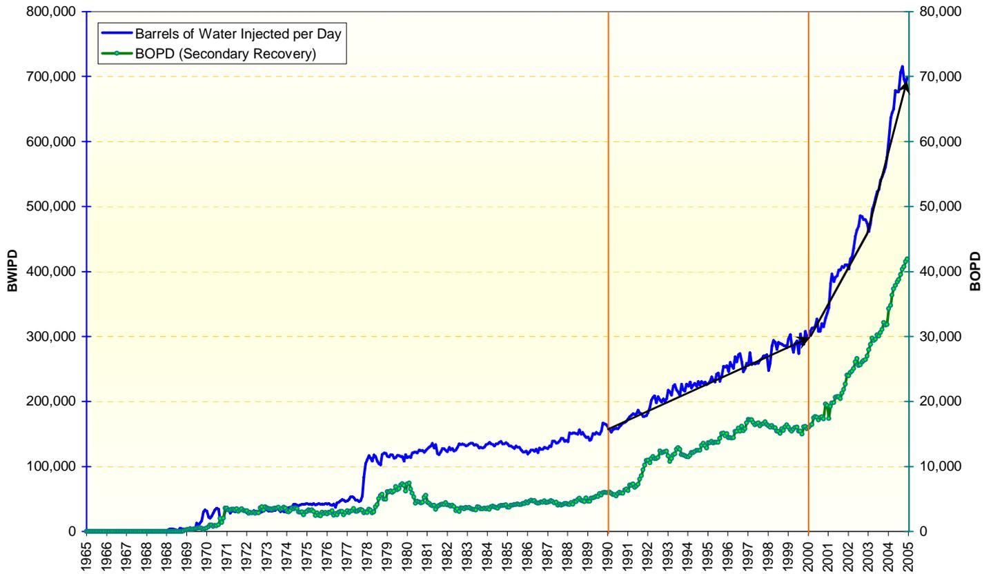
Fig. 1 – Injected water and secondary recovery oil production
