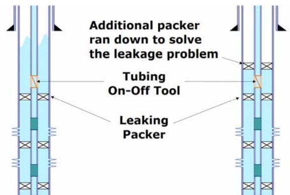
Fig. 12 –.Advantage of having an on-off tool above the selective installation
