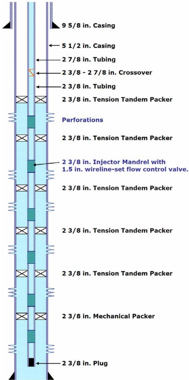
Fig. 4 – Mechanical Packers Completion
