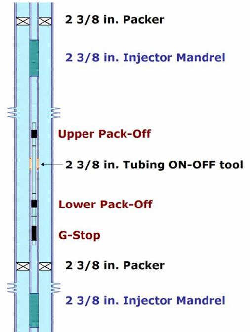
Fig. 11 –Patching of an on-off tool leakage.
