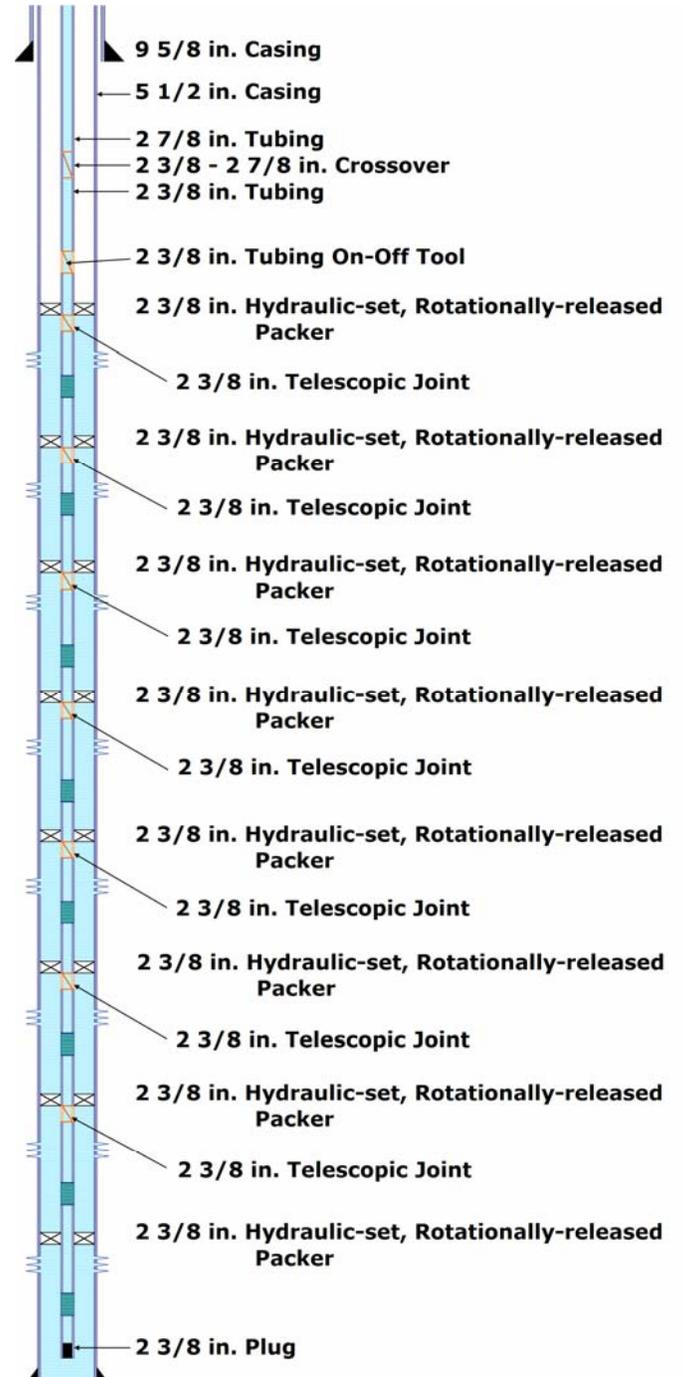
Fig. 9 – Hydraulic-set rotationally-released completion with telescopic joints
